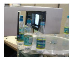
The 51R55 is a conveyer-based system that uses three Point Grey 1024x768 RGB color Flea2 cameras, placed 180 degrees from each other, to provide a 360 degree inspection of a plastic bottle's cap tamper band. In addition to checking that the tamper band has no
