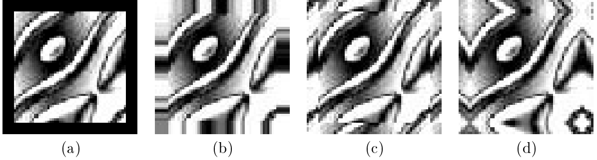
Figure 2: Image extension for R = 5 : (a) zero padding, (b) constant replication, (c) periodic replication, (d) mirror replication
