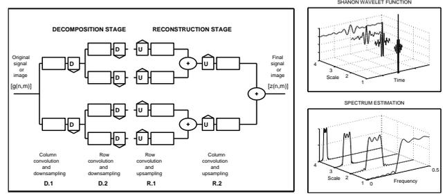
Figure 3: Wavelet transform use in signal decomposition and the effect of Shannon wavelet function dilation to its spectrum compression
