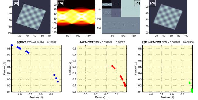
Figure 6: Figure presents (a) rotation of simulated image, (b) its Radon transform, (c) decomposition of the Radon transform image into 2. level, (d) inverse Radon transform of (b) and below comparison of image features evaluated by methods mentioned in text before
