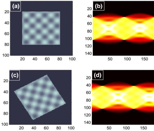
Figure 5: (a) Simulated image sample and (b) its Radon transform. (c) Rotated simulated image by angle  $\Theta = 30^\circ$  and (d) its Radon transform. The translation effect is a translation along  $\Theta$  (horizontal axis here)
